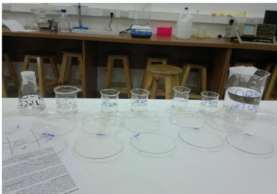
Figure 3.1: Swelling test for SF biofilms with ABS and PBS.
